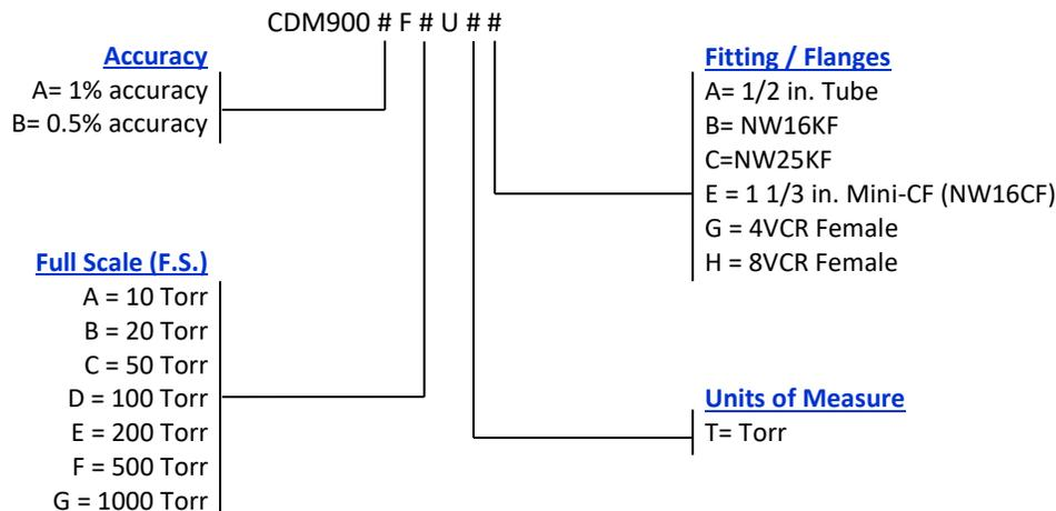
Example: CDM900BFAUTB (CDM900, 0.5% accuracy, 10 Torr F.S, Torr units of measure, NW16KF fitting)
