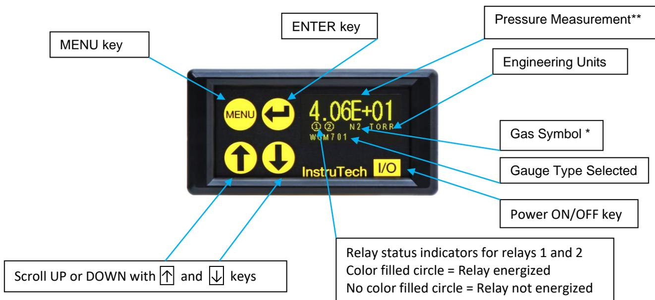
\* If you are using gas dependent gauges such as the WGM701, CCM502, etc., on gases other than air/nitrogen you must manually apply correction factors to the pressure readings per instructions given in the user Manuals of these devices.
