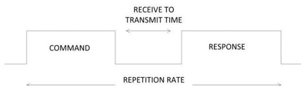
The maximum command repetition rate will depend on the length of the command sent and the response received, as well as the baud rate. The maximum repetition rate for the baud rate you are using can be found in the following table:
