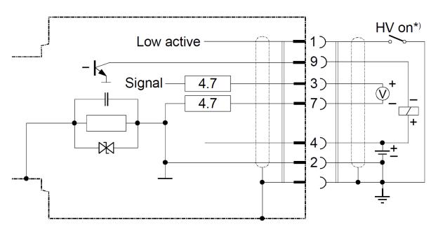
\* Does not apply to WGM701. Pin 1 is not assigned. Digital input to gauge is not required as high voltage for cold cathode sensor is turned on automatically once measurements from pirani has indicated low enough pressure level.
