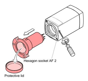
WARNING! Helium may cause electric arcing with detrimental effects on the electronics of the product. Before performing any leak tests disconnect power and remove the electronics unit.
