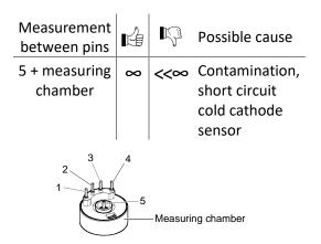
Replace measuring chamber if defective.
