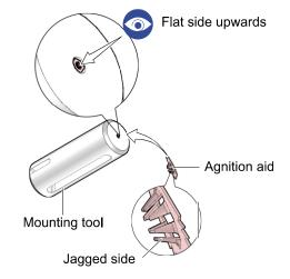
... and slide it onto the anode until the stop position is reached.
