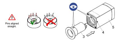
• Fasten the measuring chamber (3) by means of the hexagon socket set screw (4).
