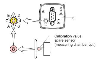
• Carefully slide the measuring chamber (3) into the electronics unit (5) until the mechanical stop is reached.
