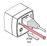
✓ If the output from the gauge corresponds to 760 Torr, the ATM adjustment has been successful. Otherwise, repeat the adjustment procedure.
