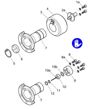
The parts can now be cleaned or replaced individually as described in the section 6.7.
