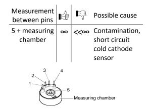
Replace measuring chamber if defective.
