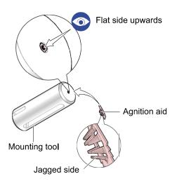
... and slide it onto the anode until the stop position is reached.
