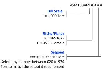
Example: VSM100AF1G030 (Absolute vacuum switch with 4VCR fitting, setpoint at 30 Torr)
