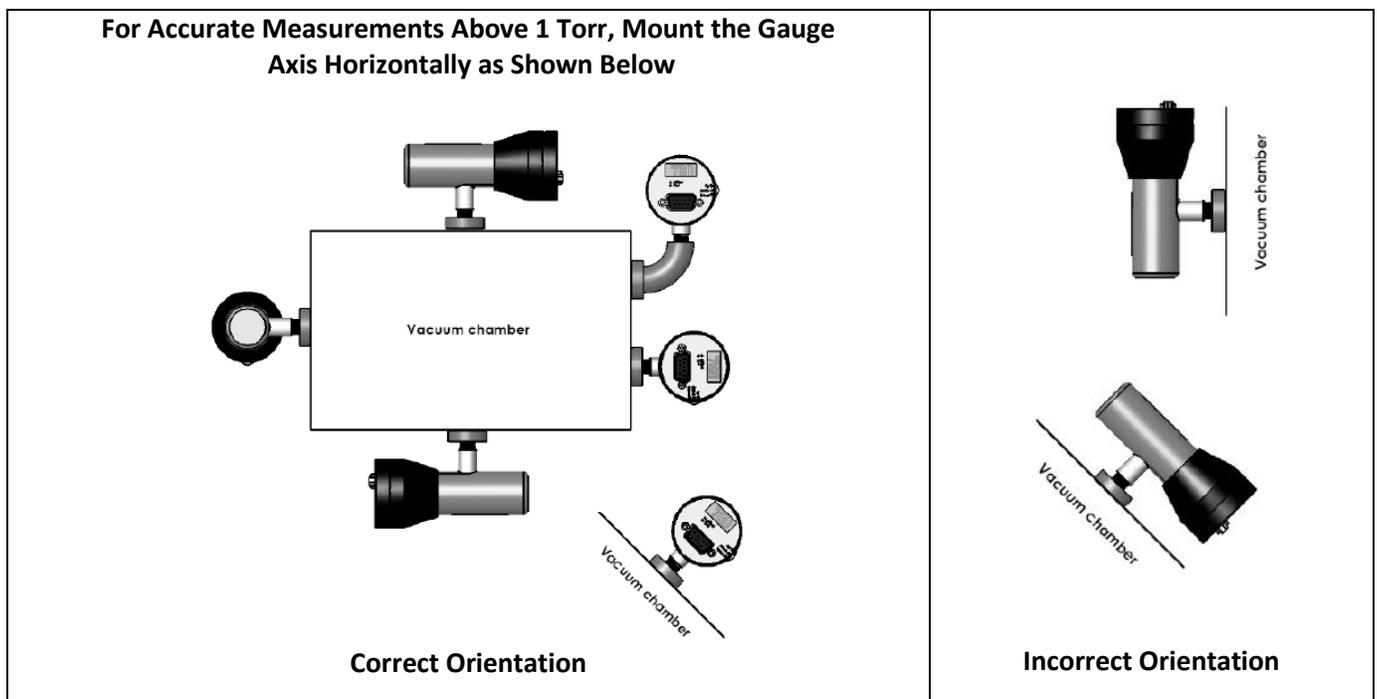
Mount the CVM211 with port down, if possible, to help minimize the effect of any particles or condensation from collecting in the gauge.
