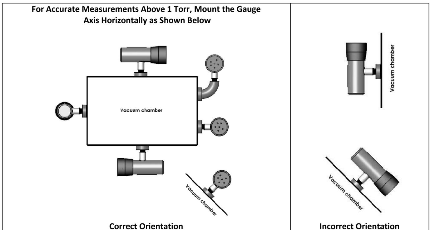
Mount the CVG101 with port down, if possible, to help minimize the effect of any particles or condensation from collecting in the gauge.
