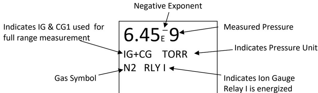
**Ex 3A: IG + CG1 data displayed for full range vacuum measurements with CG1 in IG + CG1 LG mode**
