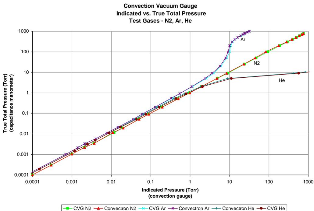
The Y- Axis is actual pressure, measured by a capacitance manometer, a diaphragm gauge that measures true total pressure, independent of gas composition. The X-Axis is the pressure reading indicated by the convection gauge under test. The chart above shows readings for an InstruTech’s CVG101 convection gauges as well as for a Granville-Phillips® Convector® gauge, to illustrate that the response of both these type of gauges is virtually the same.
