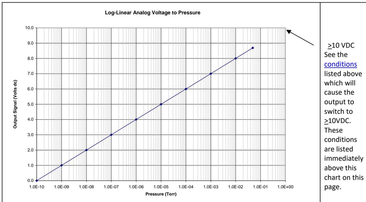
**6.2 Ion gauge plus convection gauge analog output - IG + CG1**
