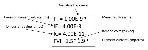
Example - R&D Display of Critical Hot-Cathode Ion Gauge Measurement Parameters
