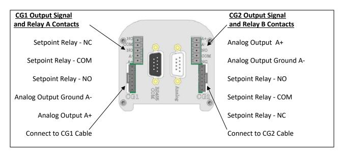
IGM402 I/O Terminal Blocks for CG1, CG2, RELAY A and RELAY B
