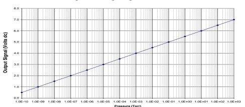
Log-Linear Analog Voltage to Pressure
