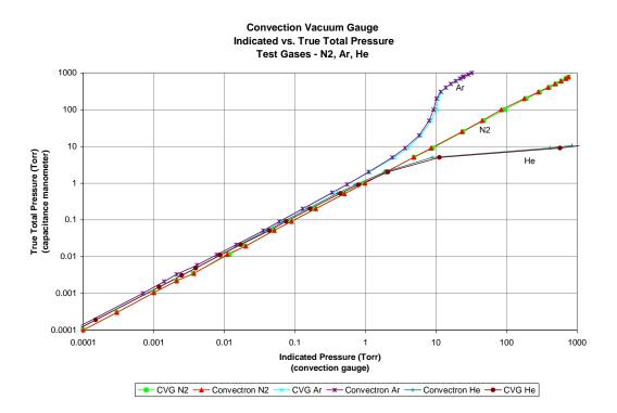
The Y- Axis is actual pressure, measured by a capacitance manometer, a diaphragm gauge that measures true total pressure, independent of gas composition. The X-Axis is the pressure reading indicated by the convection gauge under test. The chart above shows readings for an InstruTech's CVG101 convection gauges as well as for a Granville-Phillips<sup>®</sup> Convectron<sup>®</sup> gauge, to illustrate that the response of both these type of gauges is virtually the same.
